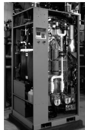
Photo 1 5 kW SOFC System
